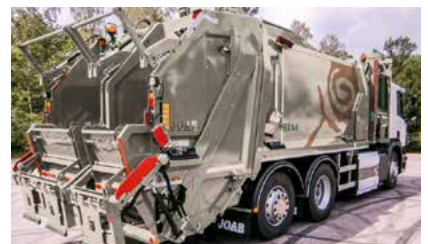
Rear loader with two chambers (paper + plastic).
