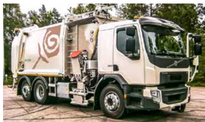
Side loader with two chambers (waste + bio).
